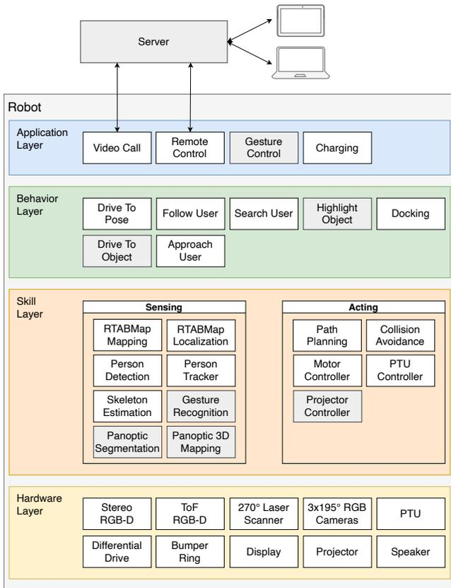
Fig. 3. Software architecture for the CO-HUMANICS robot companion. Modules in gray boxes are in development and not yet fully integrated.
