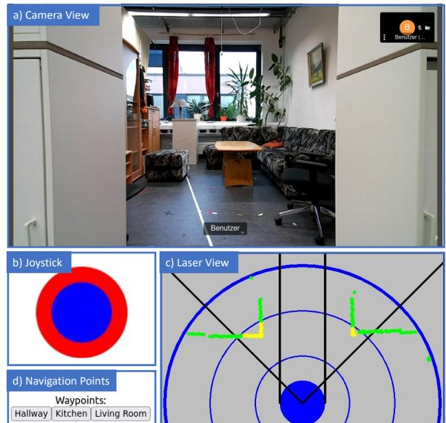
Fig. 6. Current prototype of the user interface of the virtual guest: a) current camera view, b) virtual joystick to send drive commands, c) corresponding top view of local laser measurements (yellow and green depending on distance) with range circles and dimension of the robot and d) predefined positions to let the robot navigate to.
