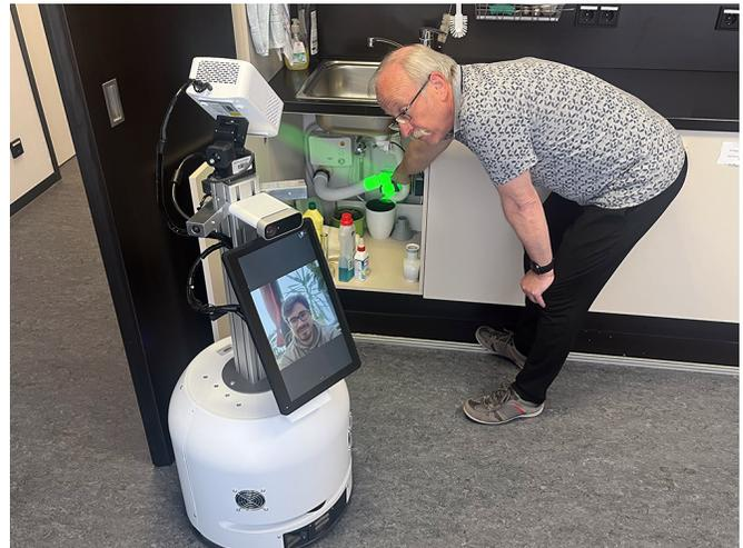
Fig. 1. The CO-HUMANICS robot companion enables a virtual guest to remotely assist an older adult in a repair task by highlighting a pipe in the video call with the projector.
