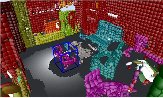
Fig. 5. Panoptic NDT map of a real apartment with a 3D bounding box highlighting a chair selected as target for robot navigation. The robot respects the chair's orientation as visualized by the cost function (ground plane): white indicates optimal while black indicates least optimal. Panoptic labels are visualized by small color differences based on the semantic colors: red - wall, yellow - cabinet, purple - chair, cyan - sofa, gray - table, orange - tv.
