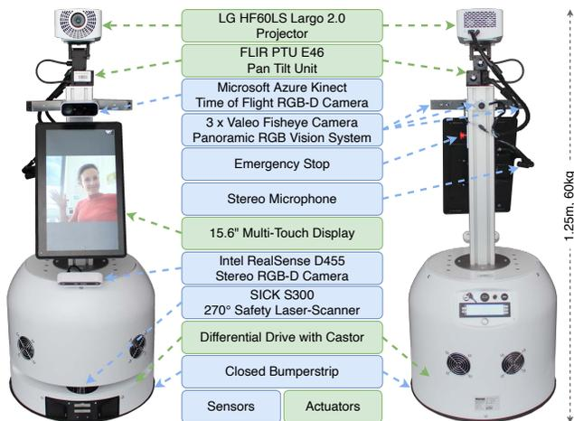
Fig. 2. The CO-HUMANICS robot companion with its sensors (blue) and actuators (green).
