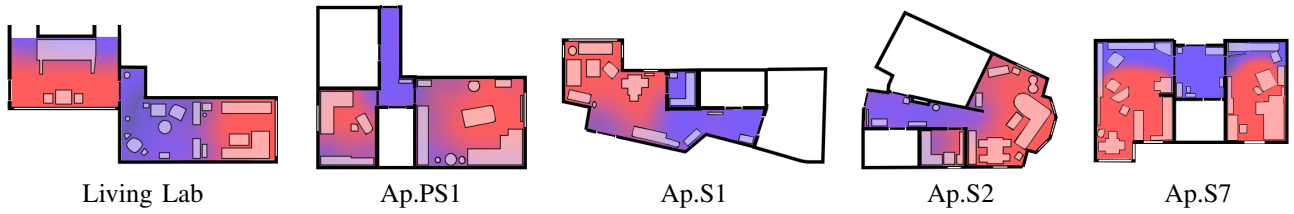
Fig. 4: Layout of our test apartments: the robot operated in the colored regions only; obstacles are restricting the operational area for the robot additionally; red color is indicating areas with incidence of daylight, blue of artificial light.
