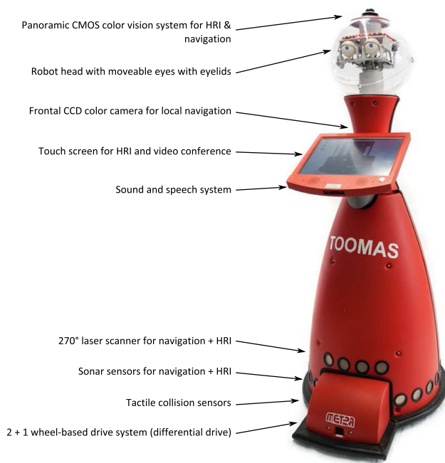
Fig. 1 Interactive mobile shopping robot TOOMAS based on a SCITOS A5 (developed by MetraLabs GmbH Ilmenau, Germany) with its main equipment for environment perception, navigation, and human-robot interaction
