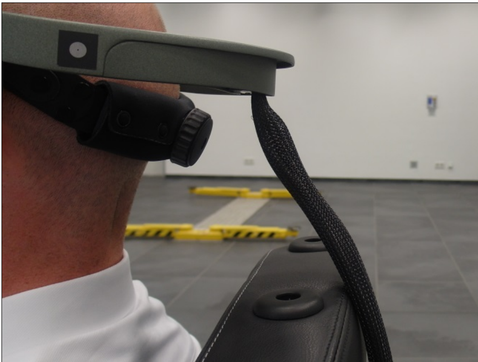
Figure 2: Cable routing of the NVIS nVisor ST50 HMD.
